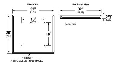
**General:** Furnish and install as shown on plans DURAPAN" Wash Machine and Water Heater Pan, Model 98, as manufactured by E.L. Mustee & Sons, Inc. One-piece compression molded fiberglass using matched metal molds under extreme heat and pressure. Shoulder will be no less than 2½" high. Removable aluminum threshold with water tight seal secured by stainless steel screws. May be secured to sub-floor; mounting hardware provided. Shall include (1) 1 "NPSM-90° elbow fitting. Color: White.
